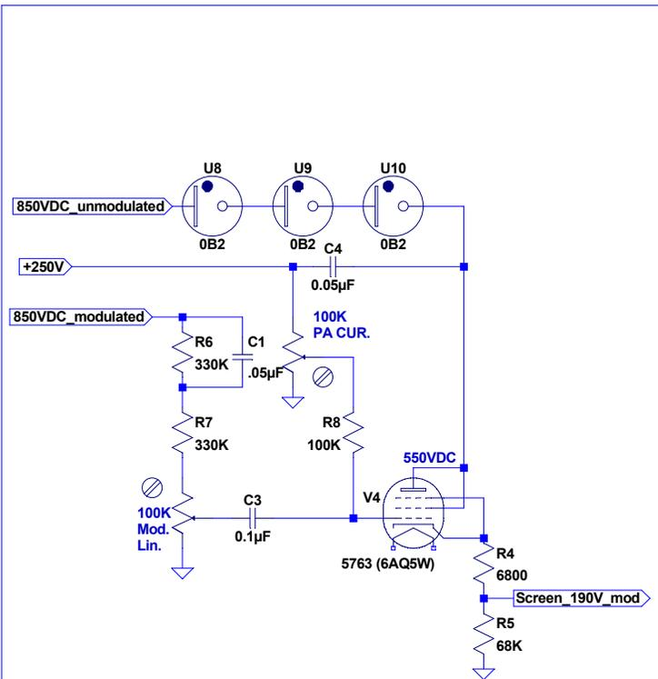
Screen modulator from T-282(\*)/GR transmitter. Three 4X150As are plate modulated. R4 is tuning voltage screen dropper. Short R4 for "Operate" The small complexity is used instead of a separate screen modulation winding on the modulation transformer. The advantage is that the carrier-level screen voltage and the level of modulating voltage can be set for best linearity.
