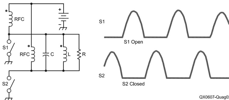
Figure 2 — Basic waveforms.
