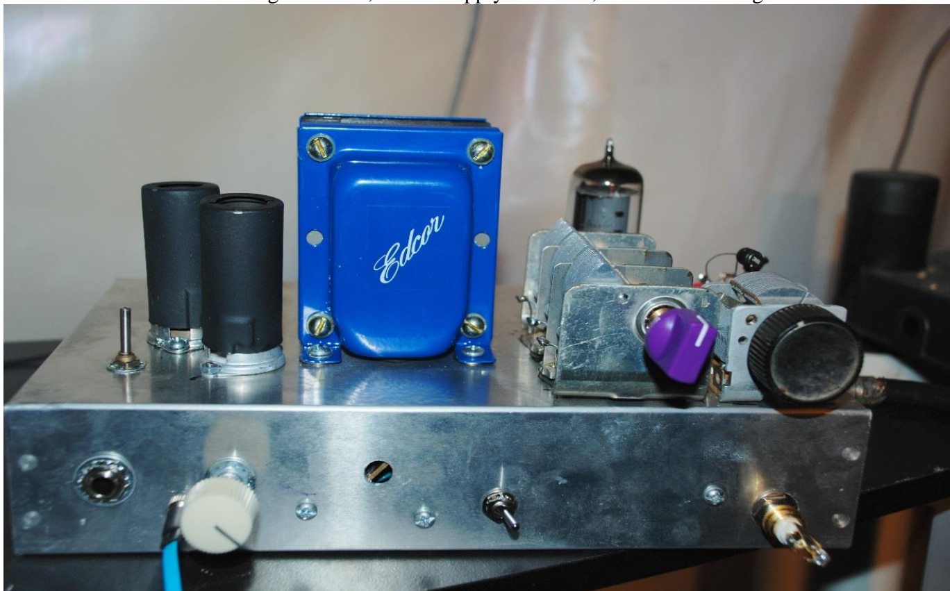
Audio Stages on Left, Power Supply in Center, RF section on Right
