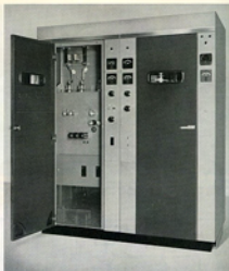
FIG. 2. The anode and UFA stages are shown here. Note the three crystal sockets on the carrier chassis, and the way to reach tubes.
