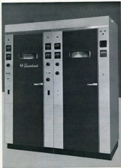
FIG. 1. Easy access to all tubes is made through two interlocked front doors of the RIA-5T Transmitter. The PA, modulator, and antenna modulators are in the cabinet on the right, and the exciter, driver and control equipment is on the left. The attractively styled cabinets are available with red or gray doors.
