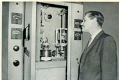
FIG. 4. The author is shown adjusting the new FA stage. Only one 17A2 tube is used for high efficiency operation. The coil, shown on the right, is the third harmonic coil used in the plate circuit of the FA to increase efficiency by shaping the plate waveform.
