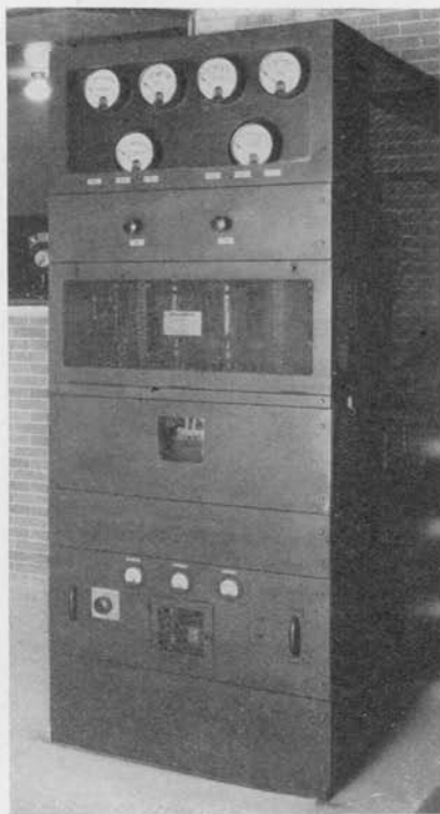
Fig. 9—Class B modulator unit at KDKA.
