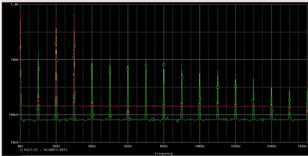
The RMS demodulator (red) is still a low distortion one, the ideal ENVELOPE demodulator maintains its distortion prone behavior.
