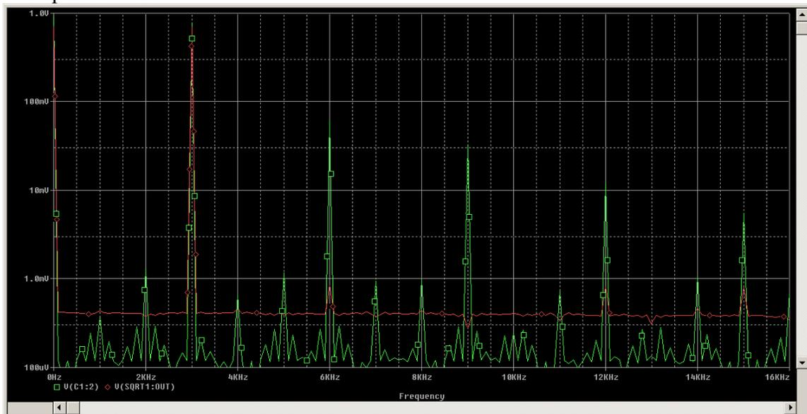
The RMS demodulator is superior to the envelope demodulator. In fact the second harmonic at 6 kHz is less than 20 dB down in the envelope demodulator (green), it is almost negligible in the RMS demodulator (red).
