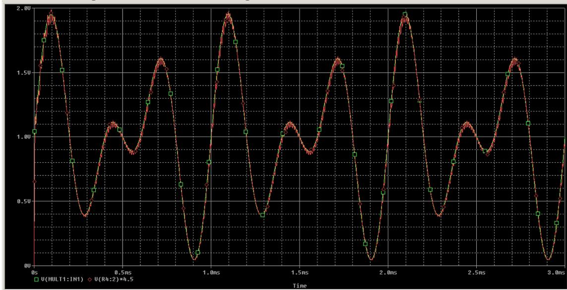
The superposition is almost perfect if losses of the phasing network are compensated by a scale factor of 4.5. Some residual ripple is caused by imperfections of the phasing network, that has been optimized by successive approximations.
