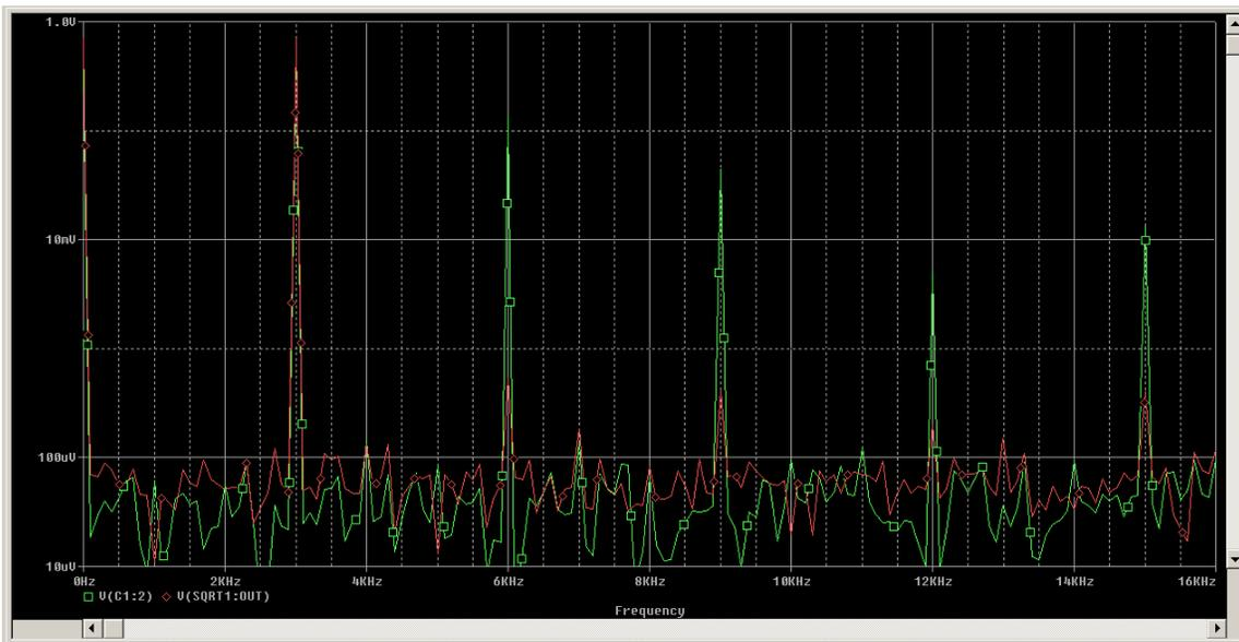
Harmonic distortion is again very high for the elementary “real” ENVELOPE demodulator (green).
