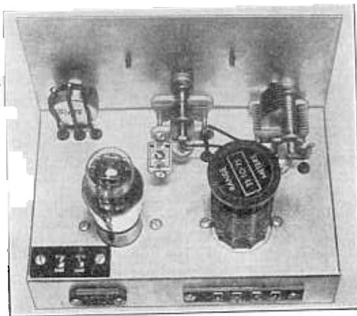
This view clearly shows the arrangement of parts for the one-tube battery set.
