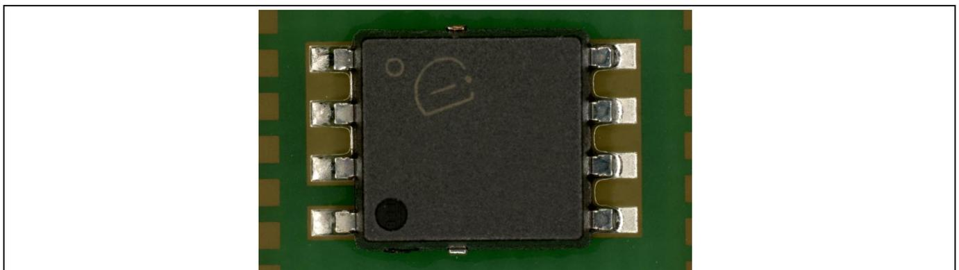
**Figure 15** Photograph of a TDSO-8 with LTI solder joints on a test board. The different appearance of the gate and source leads on the left side compared to the leads fused with the pad on the right side is visible.
