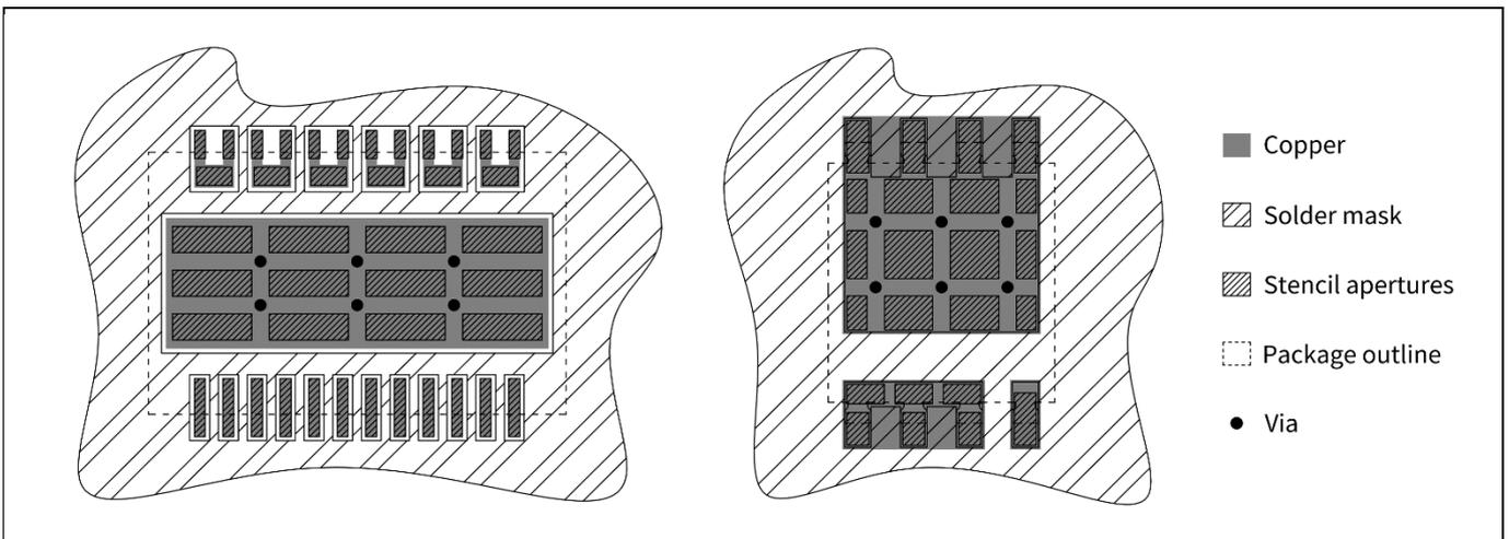
**Figure 12 Exemplary via-in-pad designs for a TSON (left) and a TDSO component (right).**
