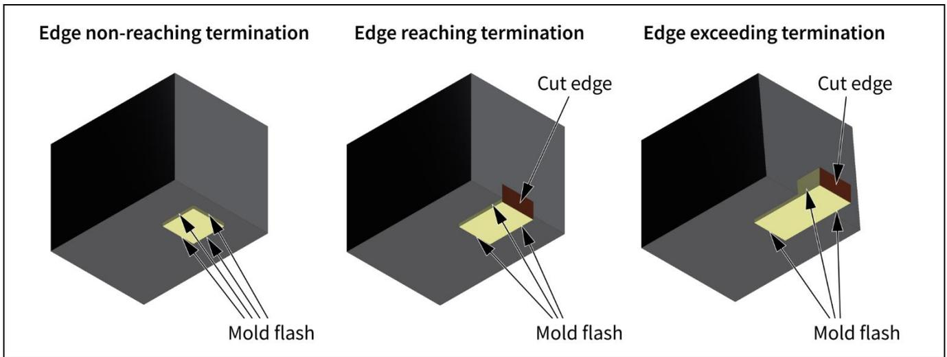
**Figure 9** Models of the basic termination types with wettable areas on bottom only. Cut edge areas and such covered with mold flash are considered to be non-wettable by design.
