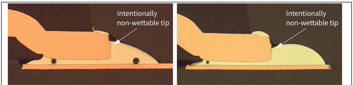
**Figure 6** Cross sections of TDSON-8 without LTI. The wetting behavior on the cut edge is inconsistent.
