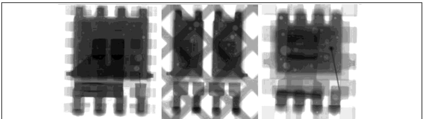
**Figure 17** X-ray photographs of properly a soldered TDSON-8 (left), a TDSON-8 with dual pad (center), and a TSDSON-8 (right).
