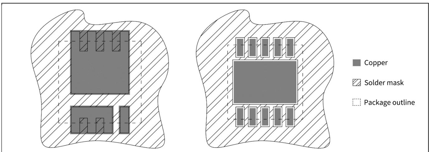
**Figure 8** Example of SMD pads for a TSDSON-8 power package (left) and of NSMD pads for an USON-10 package (right).
