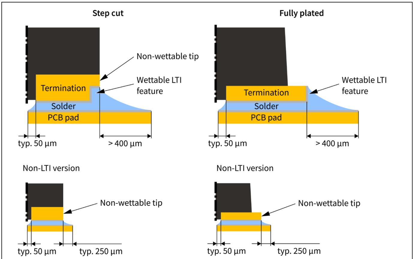
**Figure 11 Schematic comparisons of a “step cut” LTI example with partial leadframe thickness wetting height, and a “fully plated” LTI example with full leadframe thickness wetting height. For comparison, non-LTI examples are shown (lower 2 illustrations). For complete LTI functionality, a distinct solder meniscus must be formed at the termination tip by sufficient extension of the pad over the package edge.**
