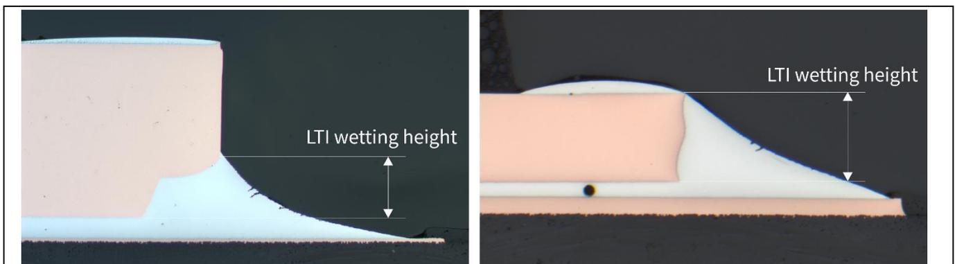
**Figure 7** Cross section of a soldered trapezium groove LTI on the HSOF-8 (left) and of a soldered fully plated LTI on the TDSON-8 (right).
