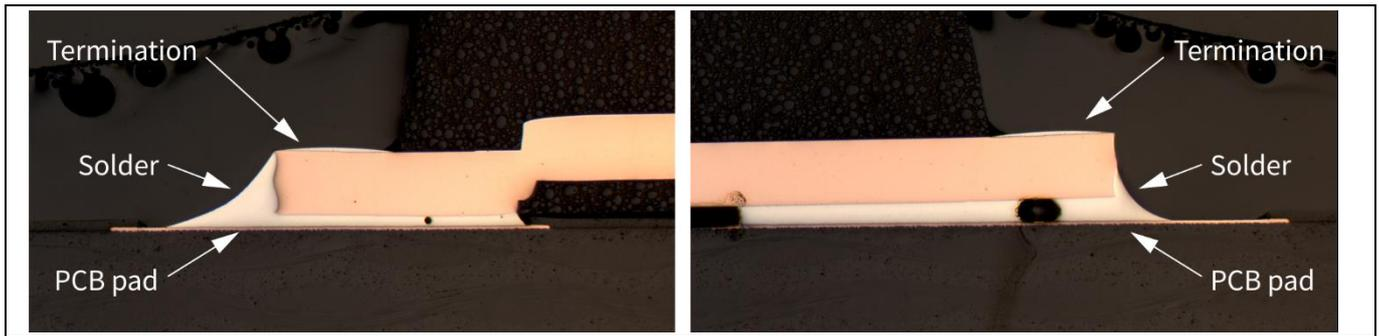
**Figure 16** Cross section of a TDSON-8 assembled on board. The natural tilt of the package is visible causing the different appearance of the solder joint fillet on leads that are fused with the pad (right) compared to the single ones (left). However, the LTI tips are wetting properly on both sides.
