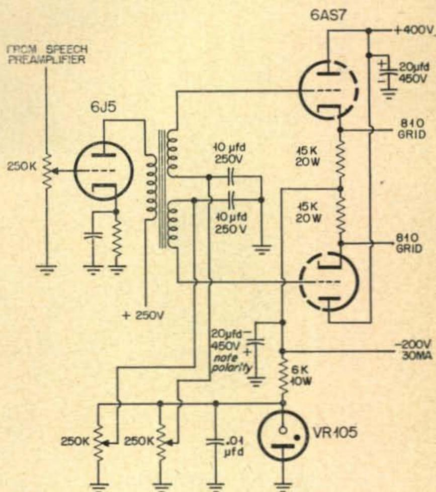
peak power demand of . . . call it 45 watts. To handle a Class-B grid-type load, we should have some swamping load on it, and negative feedback, so that means . . . hmmm. Now look; let's not be silly! A hundred-watt transformer is a modulator transformer itself, not a *driver* transformer! No wonder we had Gravel Gertie at the mike!
