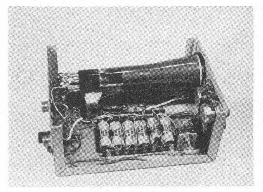
The row of electrolytics with associated diodes make up the high voltage supply. The mini-ductor on the back panel is L1 and L2 is the single turn of wire with white insulation.
