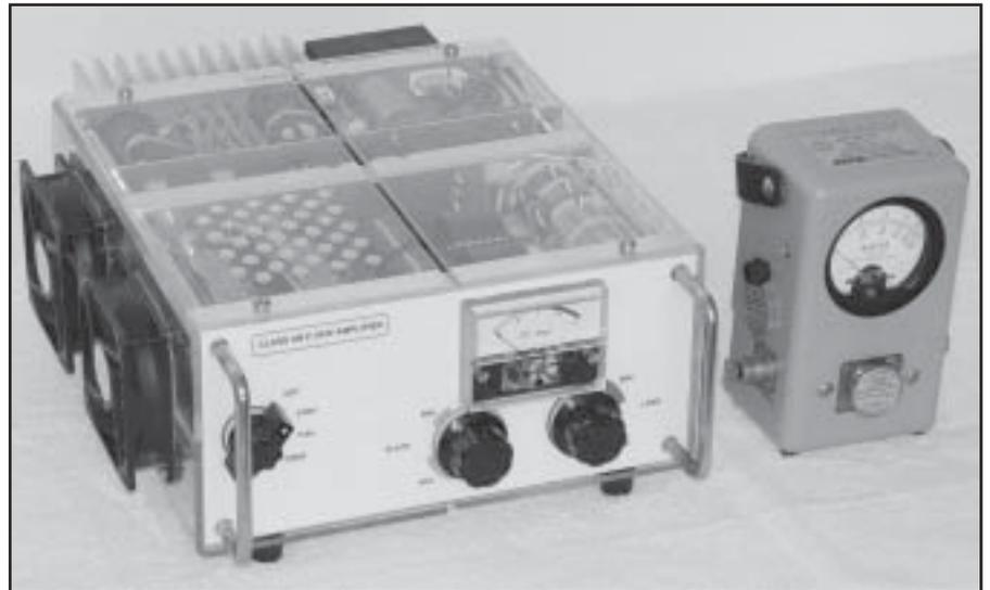
You can see the small size by comparing the amplifier to a Bird model 43 wattmeter.
