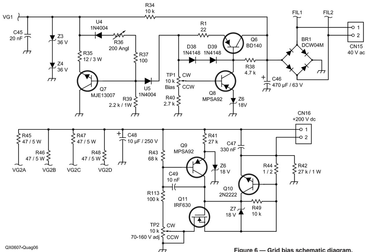
Figure 6 — Grid bias schematic diagram.
