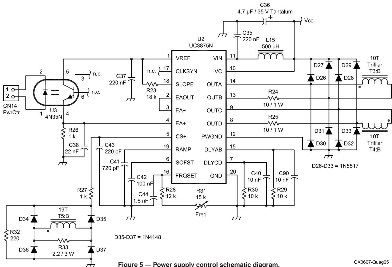
Figure 5 — Power supply control schematic diagram.
