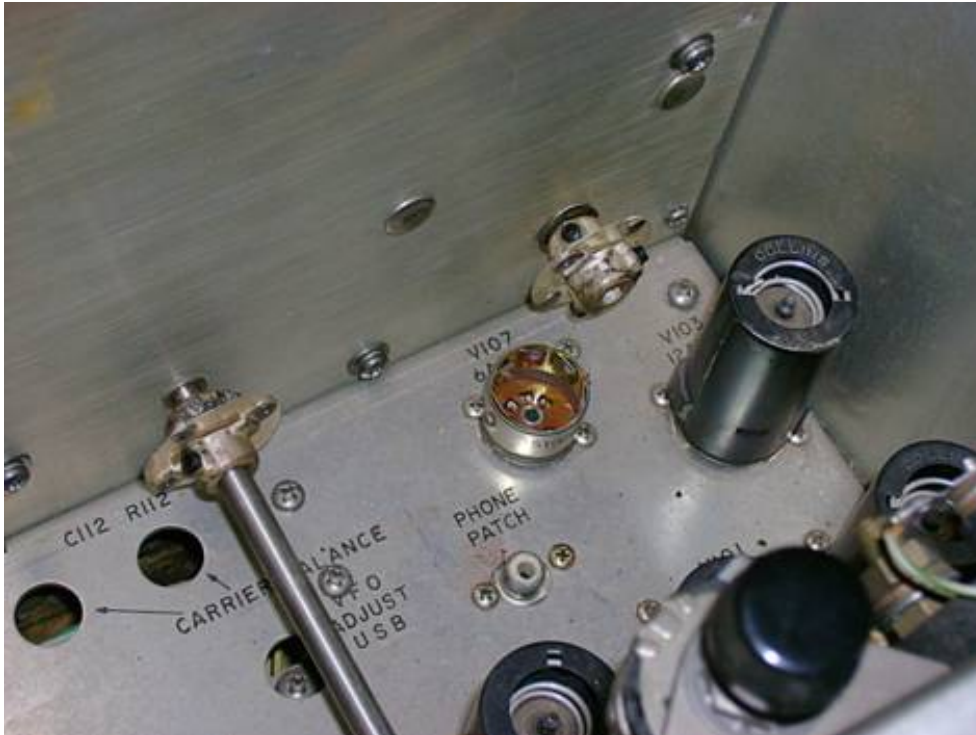
The shafts coming through the PA section with the stock couplers
