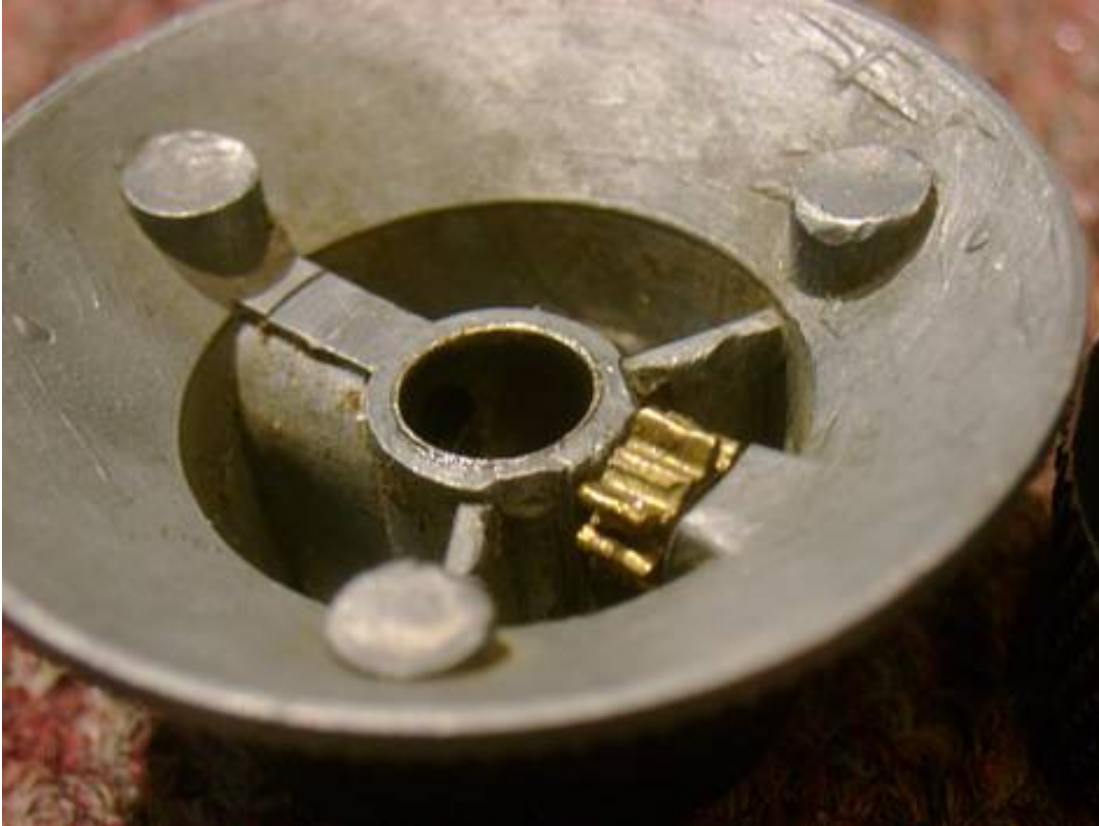
Note the worn edges, this knob it turns out had a brass insert! Note the broken brass tooth!
