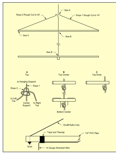
Figure 7—The rope harness is necessary for a stable hanging loop. For clarity, the knots are shown before tightening. The overhand knot is used because it holds firmly and is easy to adjust when necessary. Note that the antenna wires are fastened to the exterior of the PVC pipe.
