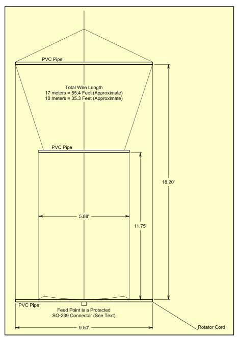
Figure 2—The rectangular loop for 17 and 10 meters.
