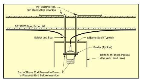
Figure 8—The feed-point connector assembly—it is a weather resistant connection that does not require taping and sealing.
