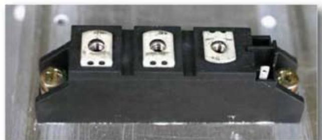
Fig. 3: Mounted device with a thickness of 60 µm thermal grease. That is a strong hint for too much thermal grease.
