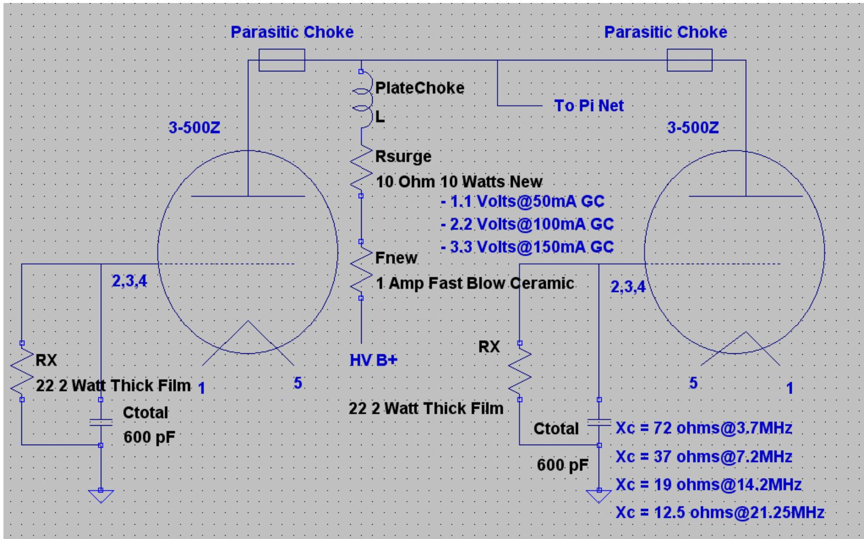
Below are some simple mods if you keep the choke circuit. The fuse in series with the Surge resistor is 2 amp fast blow ceramic that has an arc "quenching" powder in it to prevent what Carl described.
