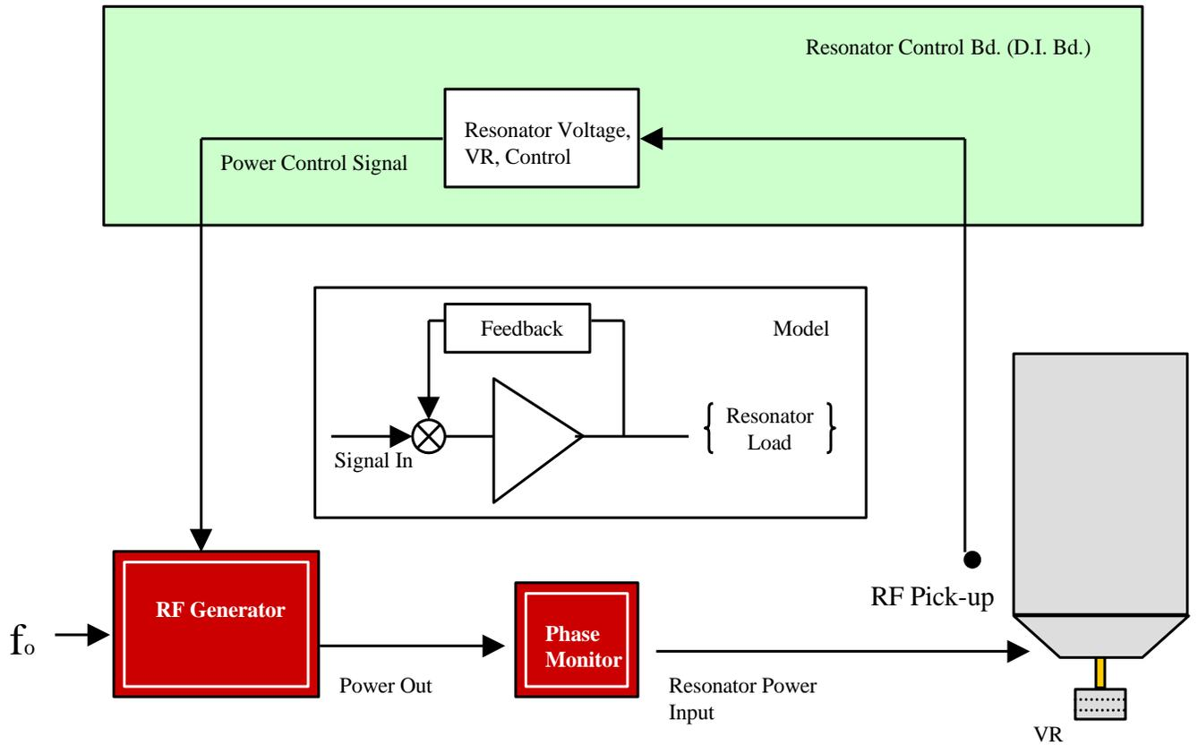
There is approximately a 1% window on the sense circuitry, which is referred to the "Set-point Status Signal" as periodically seen on the alarm window of the O/I.
