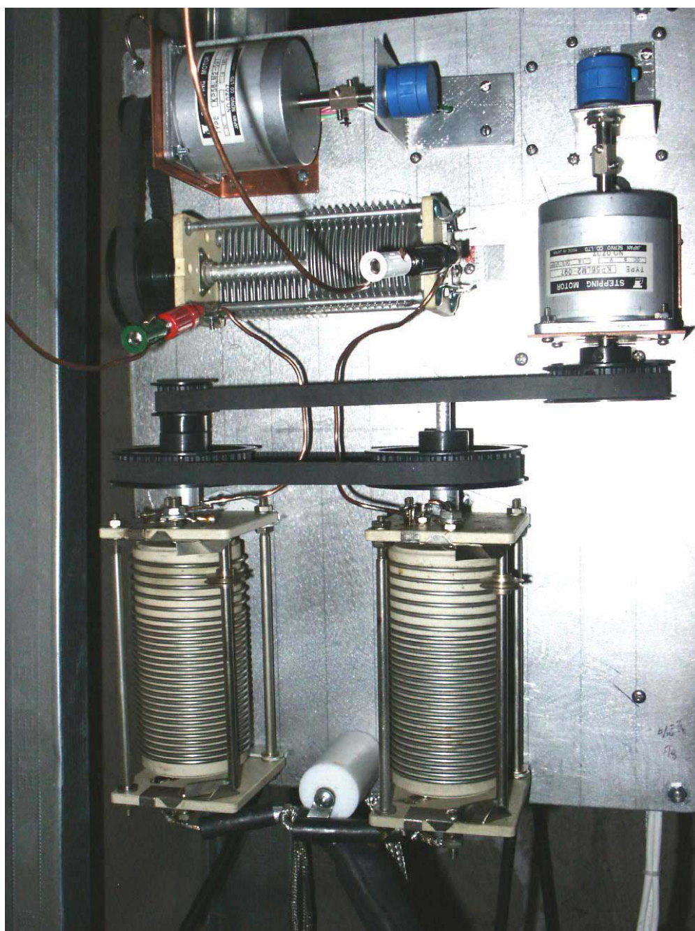
JPG of a remote controlled, balanced L-network tuner built by Mike, WA1SEO.
