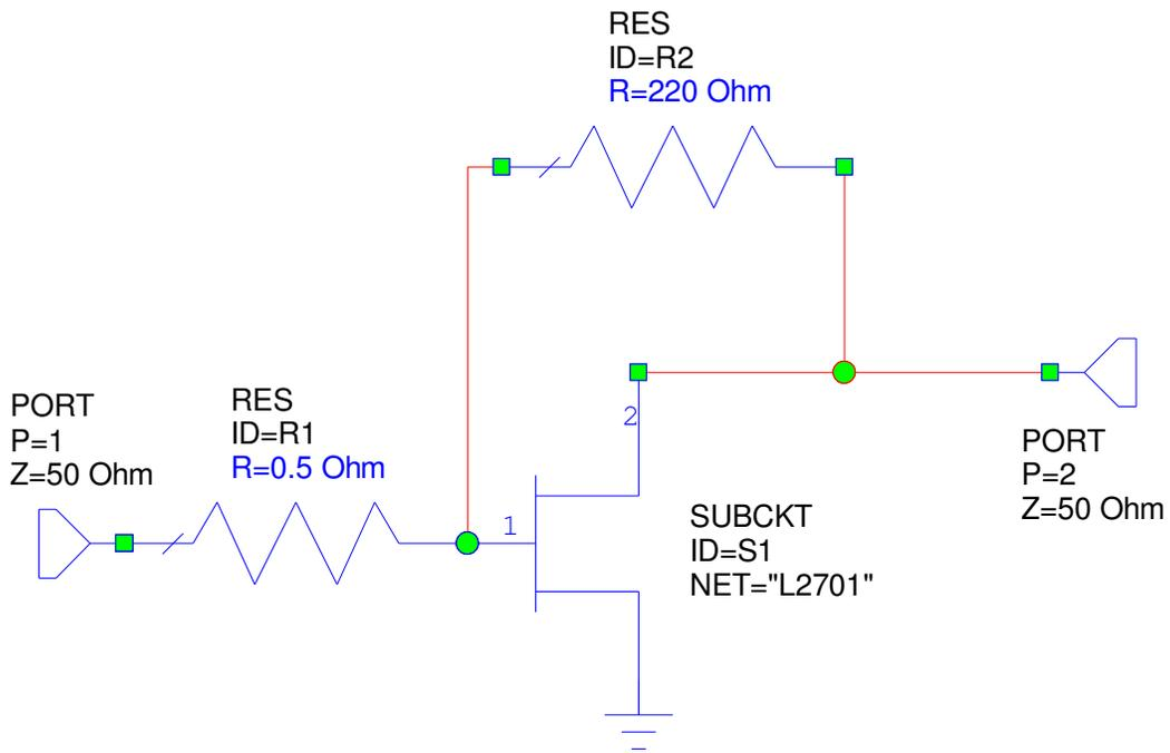
The tradeoff for this stability is to reduce the gain from 34 dB down to 17, nearly a 50 % loss. However, for this case a very equitable trade.
