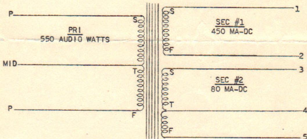
Transformer insulation tested: Pri.-8000V; Sec. #1- 11,000V; Sec. #2- 2000V to the rest of the coils and core. Primary center-tapped for Class "B" modulators. Secondary #2 will carry 80 Mills to modulate screens of beam power or screen grid tubes. Equipped with adjustable protective spark gaps on both primary and secondary.
