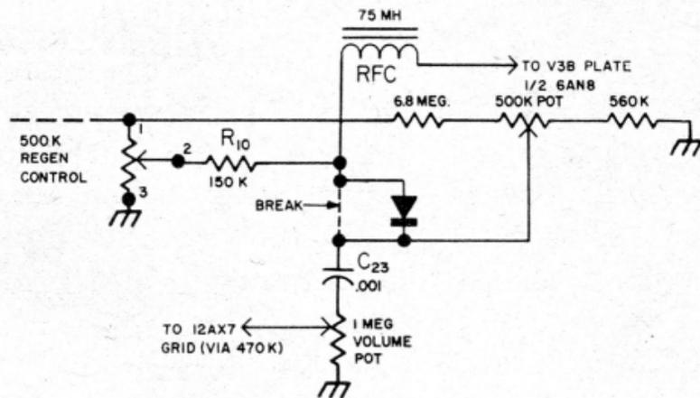
squelch should be adaptable to the older Sixer, but the resistors may have to be changed.
