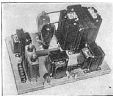
The high voltage power supply unit for use with the final amplifier of the 3-stage all-band ham transmitter.
