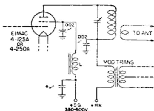
This is a sure-fire arrangement which has been thoroughly tested in the Eimac laboratory and in a number of amateur transmitters. Here a small reactor, L, takes the place of the series resistor in regard to providing a high audio impedance in the screen circuit. The d-c voltage drop inherent in the resistor method is eliminated, however, thus allowing the use of a low-voltage screen supply without requiring a three-winding modulation transformer.
