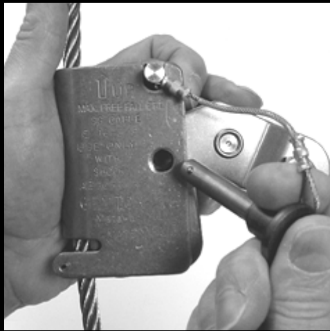
4) Close assembly, align holes and reinsert safety locking pin.
