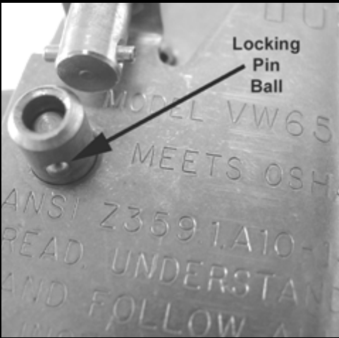
5) Make sure that locking pin balls appear on outside of main assembly.
