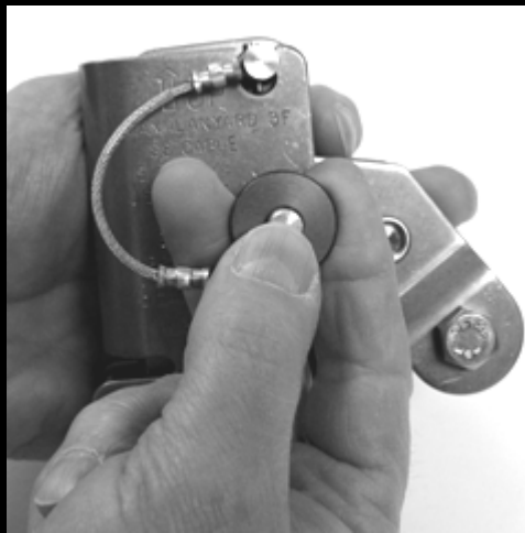
1) Depress the button on the safety locking pin and remove from main assembly
