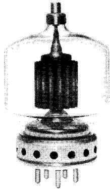
The 4-400C/6775 is a compact, ruggedly constructed, broadcast-quality tetrode having a maximum plate dissipation rating of 400 watts. It is intended for use as an amplifier, oscillator, or modulator. The low grid-plate capacitance of this tetrode coupled with its low driving-power requirement allows considerable simplification of the associated circuit and driver stage.
